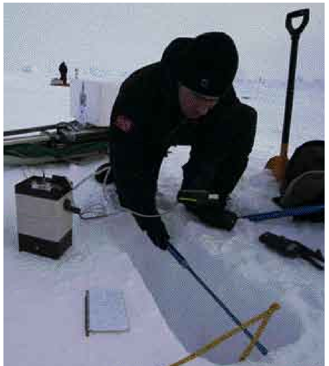
The snow's thermal conductivity is measured thanks to a heated needle. © Francis Latreille
