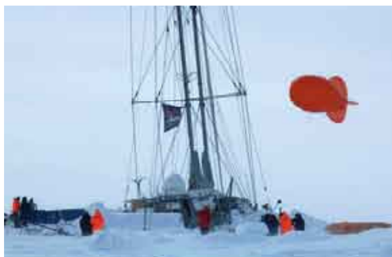
The tethered balloon can rise up to 2000 meters high to study the atmosphere © François Bernard
